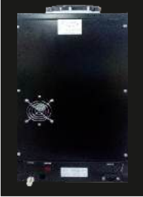
Step 1: Unplug the machine. Remove the back plate of your machine. Your machine hot tank will look like this.
